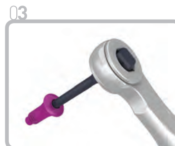
03 Place the removed abutment in the vice. Use the Ratchet Wrench to turn clockwise to separate the abutment with the Hex Remover.
